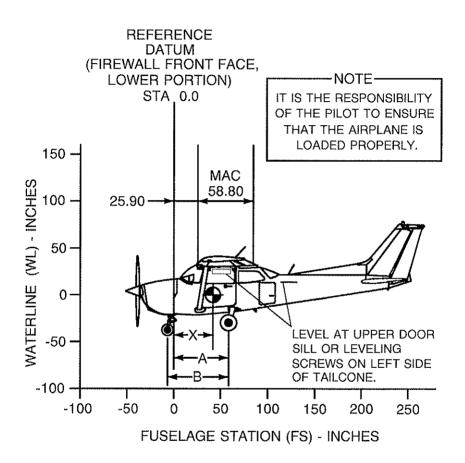
Figure 6-1. Airplane Weighing Form (Sheet 1 of 2)
