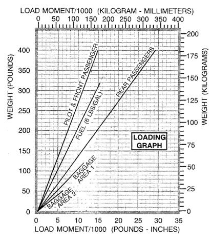
NOTE: LINE REPRESENTING ADJUSTABLE SEATS SHOWS THE PILOT OR PASSENGER CENTER OF GRAVITY ON ADJUSTABLE SEATS POSITIONED FOR AN AVERAGE OCCUPANT. REFER TO THE LOADING ARRANGEMENTS DIAGRAM FOR FORWARD AND AFT LIMITS OF OCCUPANT C.G. RANGE.
