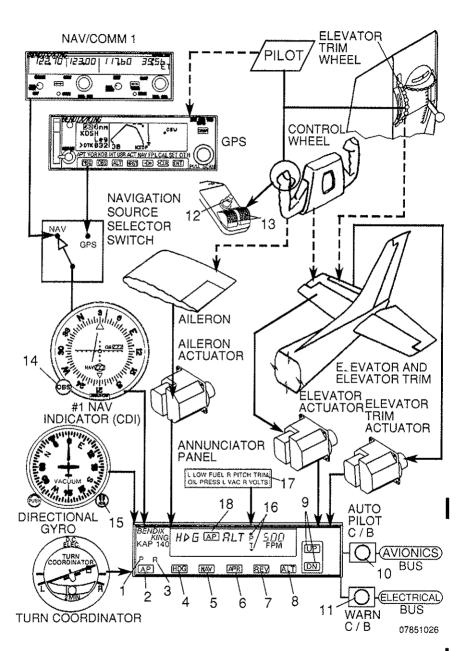
Figure 1. Bendix/King 2-Axis KAP 140 Autopilot Schematic
