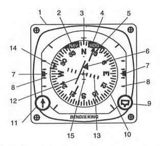
Figure 1. Horizontal Situation Indicator System (Sheet 1 of 2)
