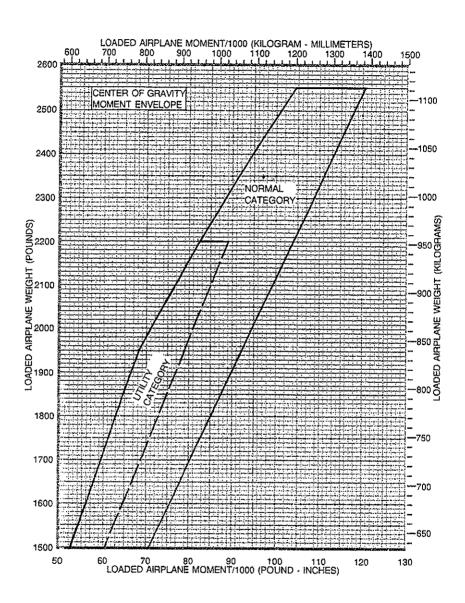
Figure 6-7. Center of Gravity Moment Envelope
