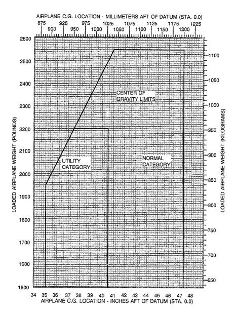
Figure 6-8. Center of Gravity Limits
